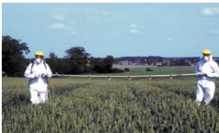
Figure 3. Application of cis -jasmone using a hydraulic spray boom in field plot trials
