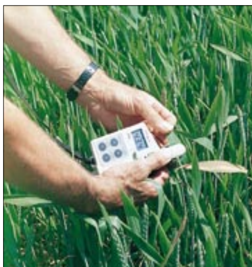
Fig. 36 A hand-held SPAD meter
