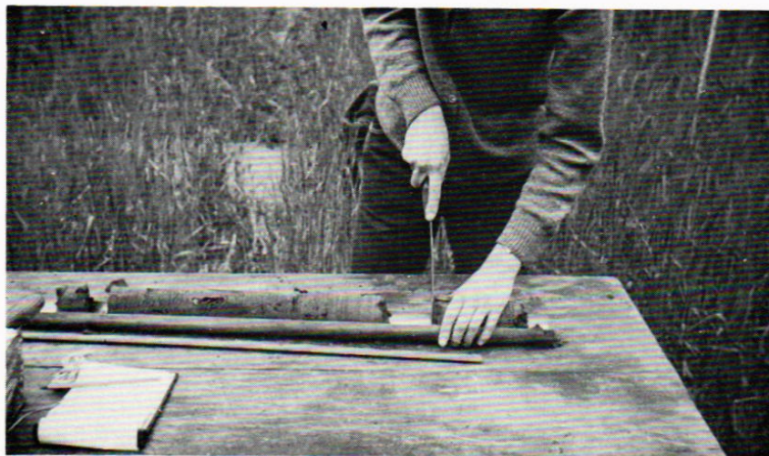
PLATE 4. Cutting core lying in a half-liner into layers.
