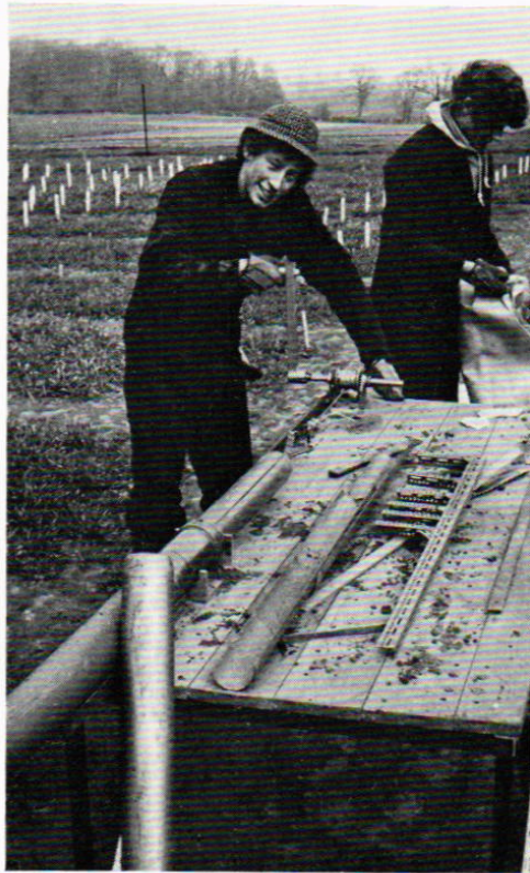
PLATE 3. Removing liners containing soil core from coring tube using hand winch.
