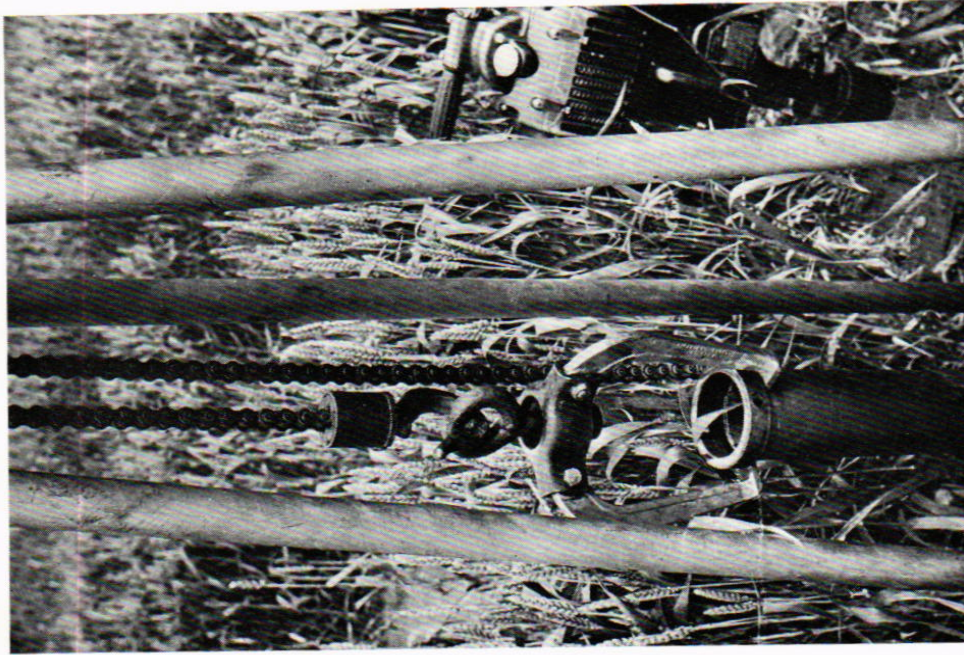
PLATE 2. Hoist and gear-puller legs attached to coring tube for lifting.
