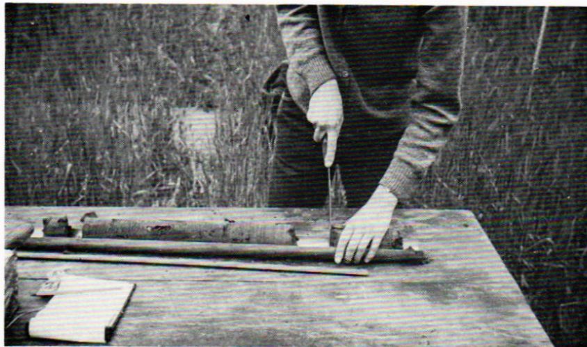
PLATE 4. Cutting core lying in a half-liner into layers.
