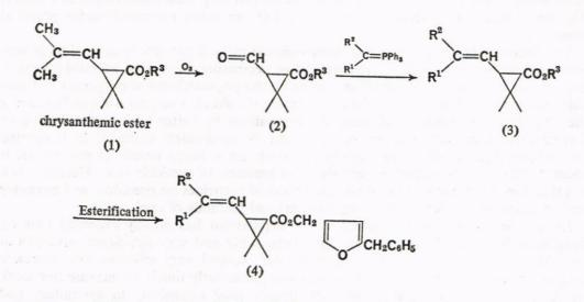
Analogues of bioresmethrin with the substituent at position 3 replaced by other groups were prepared (Fig. 1). Varying R<sup>1</sup> and R<sup>2</sup> or using other intermediates similar to those shown gave 69 esters related to (4). The most effective side chains were A, CH<sub>3</sub>. CH<sub>2</sub>. CH $\stackrel{e}{=}$ CH; B, CH<sub>2</sub>=CH.CH $\stackrel{e}{=}$ CH; C, Cl<sub>2</sub>C=CH; D, Br<sub>2</sub>C=CH (entries 3-6 in Table 1); E, CH<sub>3</sub>ON=CH.
