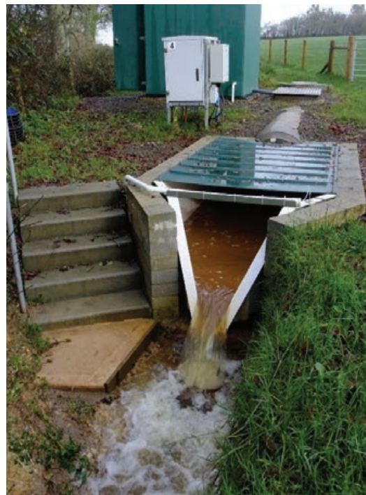
Catchment flumes and instrumentation cabin
