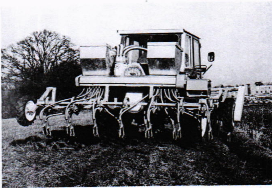
Rothamsted 'Vertical Band' granule applicator. This machine, followed by a rotary harrow, enables nematicide granules to be mixed safely and efficiently with the top 10-15 cm of the soil without harming soil structure
