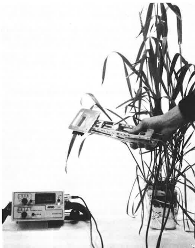
Measurement of photosynthesis and transpiration using a leaf chamber developed in the Physiology and Environmental Physics Department. The measuring system is fully portable for use on field crops.
