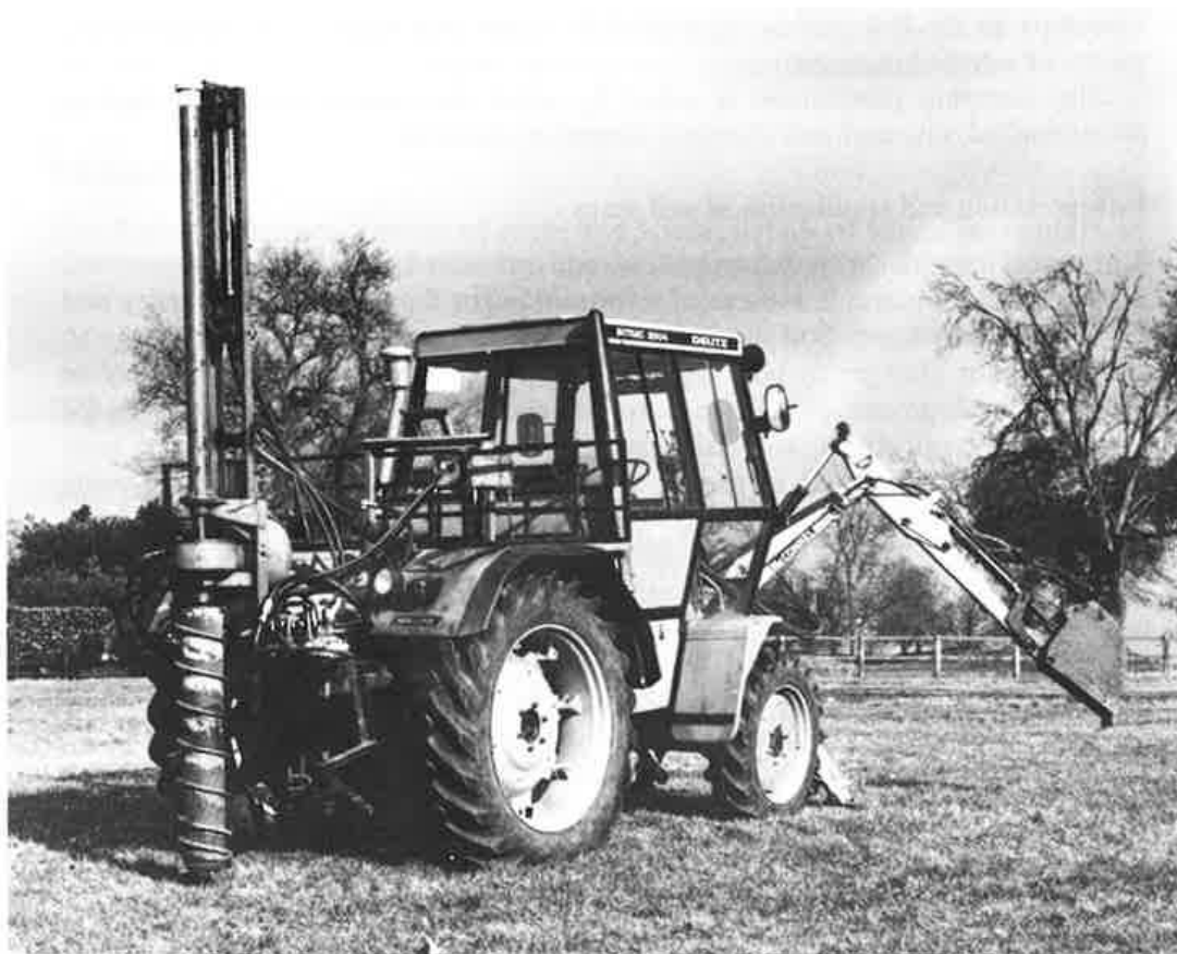
Soil corer and digger.
