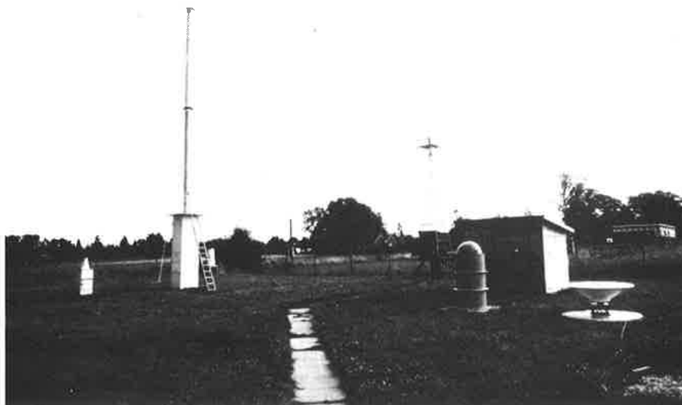
Suction trap (left) and radar set (right), with protective dome removed – two methods used for the detection of flying aphids.
