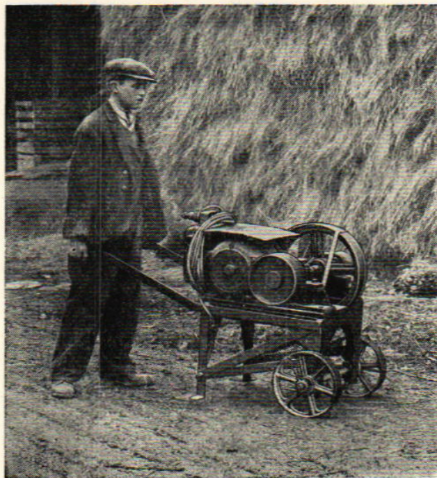
Fig. 9. 5 h.p. portable motor and countershaft on two-wheeled truck, to 7\frac{1}{2} h.p., whilst over this size, due to the greater weight, four-wheeled construction is preferable. Although the majority of designs are a combination of trucks on which the motor and control gear are mounted, there is one notable exception, namely the
