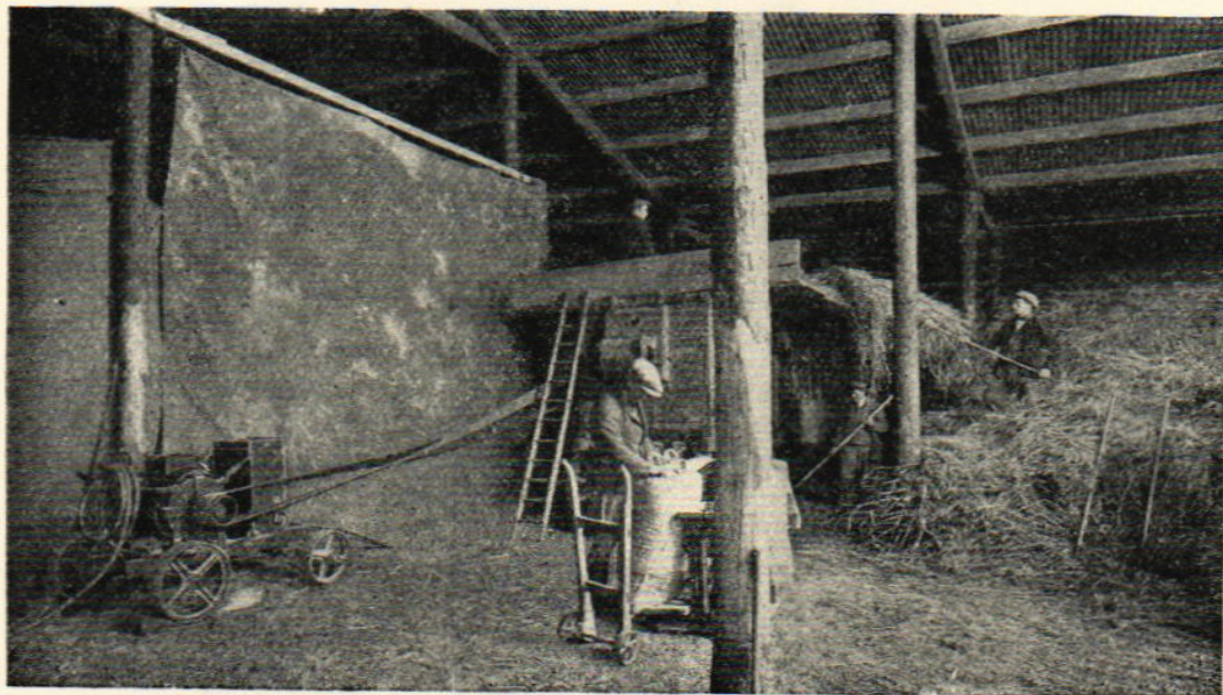
Fig. 11. 20 h.p. heavy duty portable motor driving thresher.
